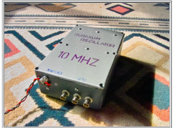
Figure 1: The portable 10 MHz Rubidium frequency reference. Click on the image for a larger version.
